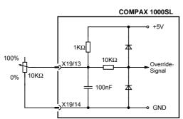
The override input is read in a cycle of 100 ms.
